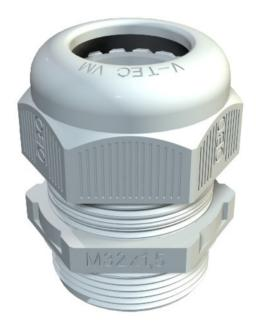
The quickest and most convenient way of providing strain relief and tightness with cable glands on junction boxes and housings is with the tried-and-trusted V-TEC VM cable glands from OBO. With the integrated sealing lip and the special OBO lamella technology protection class IP68 is achieved. Strain relief and tightness have been tested to DIN en 50262.
