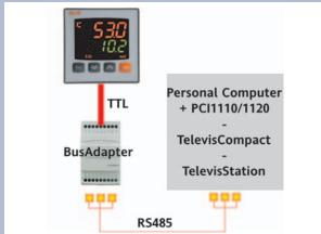
The device can be connected to Televis remote control systems through a TTL serial port (use TTL- RS interface module 485 BUS ADAPTER 150) or, in models where provided for (EW4821), by means of direct RS485 connection. To configure the device for this purpose, open the folder identified by the "Add" label and use parameters "dEA" and 'FAA".
