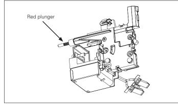
Figure 4. Remote reset interlock indicator shown.
