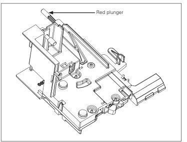
Figure 2. Non-interlocking pop-out trip indicator shown.
