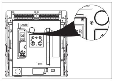
Figure 1. Installed pop-out trip indicator shown.
