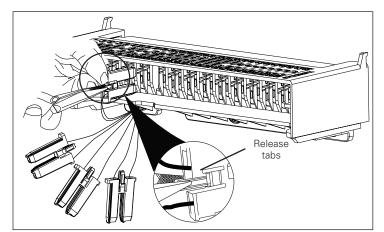
Figure 18. Connector plug removal.
