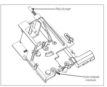
Figure 3. Interlocking pop-out trip indicator shown.
