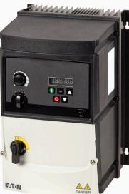
**Variable frequency drive, 400 V AC, 3-phase, 18 A, 7.5 kW, IP66/NEMA 4X, Radio interference suppression filter, Brake chopper, 7-digital display assembly, Local controls, Additional PCB protection, UV resistant, FS3**
