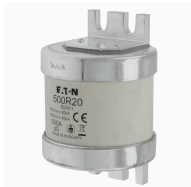
Fuse-link, low voltage, 500 A, AC 660 V, BS88, 74 x 112 mm, gL/gG, BS
