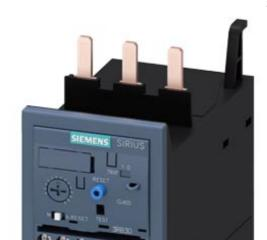
Overload relay 20...80 A Electronic For motor protection Size S2, Class 20E Contactor mounting Main circuit: Screw Auxiliary circuit: Screw Manual-Automatic-Reset
