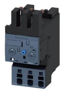
Overload relay 1...4 A Electronic For motor protection Size S0, Class 5...30 Contactor mounting Main circuit: Spring-type terminal Auxiliary circuit: Spring-type terminal Manual-Automatic-Reset Internal ground fault detection
