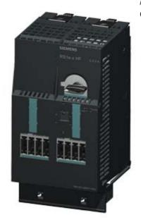
F-RS1E-X for ET 200S Failsafe reversing starter Setting range 2.4...8 A Mechanical switching Electronic protection AC-3, up to 3 kW / 400 V expandable for Brake control module 2DI module 2DI module Circuit breaker signaling parameterizable
