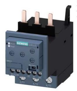
Monitoring relay, can be mounted to Contactor 3RT2, Size S2 basic, analog adjustment Apparent current monitoring 8...80 A, 50...60 Hz, 2-phase Supply 24-240 V AC/DC 1 change-over contact Monitoring for Current overshoot and undershoot Phase failure, Cable break with or without fault buffer ON delay 0-60 s Noise pulse suppression 0-30 s Switching hysteresis 6% Screw connection system
