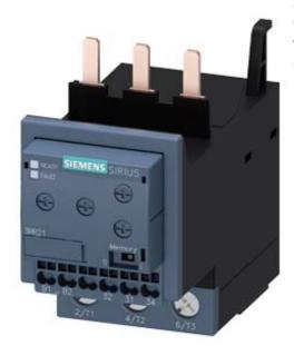
Monitoring relay, can be mounted to Contactor 3RT2, Size S2 basic, analog adjustment Apparent current monitoring 8...80 A, 50...60 Hz, 2-phase Supply 24 V AC/DC 1 change-over contact Monitoring for Current overshoot and undershoot Phase failure, Cable break with or without fault buffer ON delay 0-60 s Noise pulse suppression 0-30 s Switching hysteresis 6% spring-type connection system
