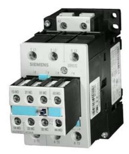
Power contactor, AC-3 40 A, 18.5 kW / 400 V 110 V AC, 50/60 Hz 2 NO + 2 NC, 3-pole, Size S2, Screw terminal !!! Phased-out product !!! Successor is SIRIUS 3RT2 Preferred successor type is >>3RT2028-1AG24<<
