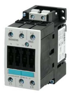
Power contactor, AC-3 40 A, 18.5 kW / 400 V 110 V AC, 50 Hz / 120 V, 60 Hz, 3-pole, Size S2, Screw terminal !!! Phased-out product !!! Successor is SIRIUS 3RT2 Preferred successor type is >>3RT2028-1AK60<<
