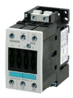
Power contactor, AC-3 50 A, 22 kW / 400 V 24 V AC, 50 Hz, 3-pole Size S2, Screw terminal Upright mounting position !!! Phased-out product !!! Successor is SIRIUS 3RT2 Preferred successor type is >>3RT2036-1AB00-1AA0<<
