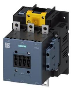
Power contactor, AC-3 115 A, 55 kW / 400 V Coil AC 50/60 Hz and DC 96-127 V x (0.8-1.1) F-PLC input 24 V DC 3-pole size S6 Auxiliary contacts 2 NO + 2 NC Main circuit: Busbar Control and auxiliary circuit: screw terminal
