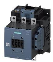
power contactor, AC-3e/AC-3 115 A, 55 kW / 400 V, Uc: 72 V DC x (0.7-1.25) PLC input 24-110 V DC 3-pole, auxiliary contacts 2 NO + 2 NC drive: electronic main circuit: busbar control and auxiliary circuit: screw terminal
