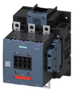
Power contactor, AC-3 185 A, 90 kW / 400 V AC (50-60 Hz) / DC operation UC 23-26 V Auxiliary contacts 2 NO + 2 NC lateral, permanently mounted 3-pole, Size S6 Busbar connections Drive: conventional
