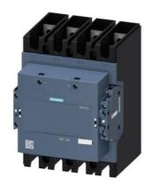
Contactor, AC-1, 350 A/400 V/40 °C, S10, 4-pole, 100-250 V AC/DC, 2 NO+2 NC, Connection rail/ screw terminal
