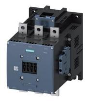
power contactor AC-1 690 A / 690 V / 40  $^{\circ}$ C 3-pole, Uc: 24 V DC (0.7-1.25) PLC input 24-110 V DC drive: electronic auxiliary contacts 2 NO + 2 NC main circuit: busbar control and auxiliary circuit: screw terminal extended rated condition railroad IEC 60077
