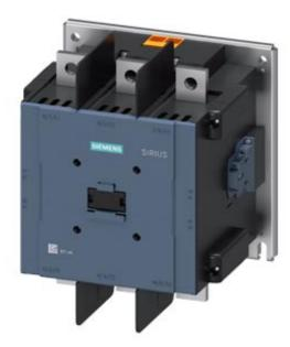
Power contactor, AC-1 1050 A, 3-pole AC (50...60 Hz) / DC operation 100...127 V AC / 100...110 V DC Operating mechanism: electronic Auxiliary contacts 2 NO + 2 NC Busbar connections Auxiliary switch and coil connections in screw-type technology
