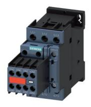
Power contactor, AC-3 12 A, 5.5 kW / 400 V 2 NO + 2 NC, 110 V AC, 50 Hz 120 V, 60 Hz, 3-pole Size S0, Screw terminal Captive auxiliary switch
