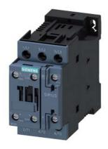
power contactor, AC-3 12 A, 5.5 kW / 400 V 1 NO + 1 NC, 24 V DC with integrated varistor 3-pole, size S0 screw terminal suitable for PLC outputs not expandable with auxiliary switch
