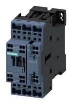
power contactor, AC-3 12 A, 5.5 kW / 400 V 1 NO + 1 NC, AC (50-60 Hz) DC operation 21-28 V AC/DC 3-pole, Size S0 Spring-type terminal
