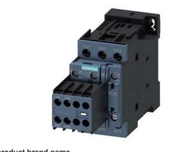
power contactor, AC-3 17 A, 7.5 kW / 400 V 2 NO + 2 NC, 24 V DC, 3-pole, Size S0 screw terminal Removable auxiliary switch
