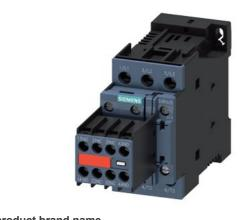
Power contactor, AC-3 25 A, 11 kW / 400 V 2 NO + 2 NC, 24 V DC, with inserted varistor 3-pole, Size S0 Screw terminal Captive auxiliary switch
