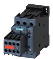
Power contactor, AC-3 25 A, 11 kW / 400 V 2 NO + 2 NC, 24 V DC, with plugged-in diode combination, 3-pole, Size S0 Screw terminal Captive auxiliary switch
