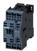
power contactor, AC-3 25 A, 11 kW / 400 V 1 NO + 1 NC, AC (50-60 Hz) DC operation 21-28 V AC/DC, 3-pole, Size S0, Spring-type terminal
