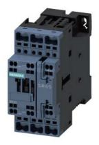
power contactor, AC-3 25 A, 11 kW / 400 V 1 NO + 1 NC, AC (50-60 Hz) DC operation 200-280 V AC/DC, 3-pole, Size S0, Spring-type terminal
