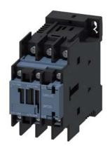
Contactor relay, AC-3 32 A, 15 kW / 400 V 1 NO + 1 NC 24 V DC, with integrated diode combination, 3-pole size S0 ring cable lug connection
