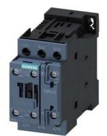
Power contactor, AC-3 38 A, 18.5 kW / 400 V 1 NO + 1 NC, 24 V DC 3-pole, size S0 screw terminals
