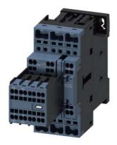
Power contactor, AC-3 38 A, 18.5 kW / 400 V 2 NO + 2 NC, 220 V AC 50/60 Hz, 3-pole Size S0, Spring-type terminals Removable auxiliary switch
