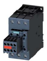
power contactor, AC-3 40 A, 18.5 kW / 400 V 2 NO + 2 NC, 230 V AC 50 / 60 Hz, with inserted varistor, 3-pole, Size S2, screw terminal Captive auxiliary switch
