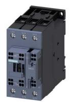
power contactor, AC-3 51 A, 22 kW / 400 V 1 NO + 1 NC, 110 V AC 50 Hz / 120 V, 60 Hz, 3-pole, size S2, spring-loaded terminal
