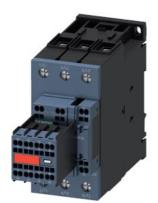
power contactor, AC-3 51 A, 22 kW / 400 V 2 NO + 2 NC, 20-33 V AC / DC with varistor, 3-pole, size S2, spring-loaded terminal, captive auxiliary switch
