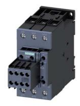
Power contactor, AC-3 80 A, 37 kW / 400 V 2 NO + 2 NC, 220 V AC 50/60 Hz, 3-pole Size S2, screw terminals
