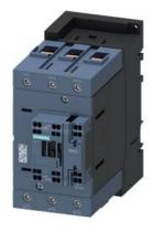
power contactor, AC-3 95 A, 45 kW / 400 V 1 NO + 1 NC, 220 V AC, 50/60 Hz 3-pole, 3NO, frame size S3 spring-loaded terminal
