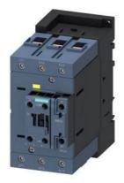
power contactor, AC-3e/AC-3, 110 A, 55 kW / 400 V, 3-pole, 21-33 V AC/DC, 50/60 Hz, with integrated varistor, auxiliary contacts: 1 NC, screw terminal, size: S3, F-PLC-IN
