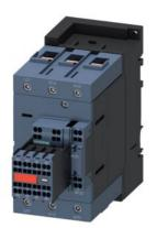
Power contactor, AC-3 110 A, 55 kW / 400 V 2 NO + 2 NC, 20-33 V AC/DC 3-pole, 3 NO, Size S3 Spring-type terminal Integrated varistor Captive auxiliary switch
