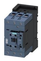
Contactor, AC-1, 140 A/690 V/40 °C, S3, 3-pole, 110 V AC, 50/60 Hz, 1 NO+1 NC, box terminal/screw terminal
