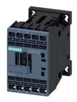
Power contactor, AC-3 9 A, 4 kW / 400 V 2 NO + 2 NC 220 V DC, 50 Hz/240 V, 60 Hz 4-pole Size S00 Spring-type terminals
