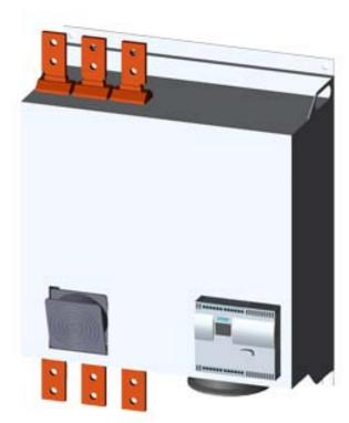
SIRIUS soft starter Values at 575 V, 50 °C standard: 1076 A, 1200 hp Inside-delta: 1864 A, 2100 hp 400-690 V AC, 115 V AC Screw terminals !!! Phased-out product !!! Successor is SIRIUS 3RW5, Preferred successor type is >>3RW5558-6HA16<<
