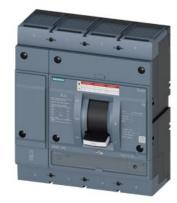
circuit breaker 3VA5 UL frame 800 breaking capacity class M 35kA @ 480 V 4-pole, line protection TM230, FTAM, In=600A overload protection Ir=600A fixed short circuit protection Ii=5...10 x In
