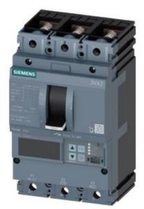
circuit breaker 3VA2 IEC frame 250 breaking capacity class L Icu=150kA @ 415V 3-pole, line protection ETU850, LSI, In=160A overload protection Ir=63A...160A short-circuit protection Isd=0.6..10x In, Ii=1.5..12x In N conductor protection optionally with external current transformer, up to 160% nut keeper kit
